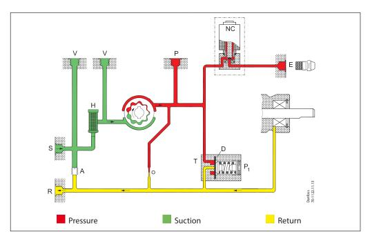
From the suction inlet (S) fuel is drawn through the filter (H) to the gear set, where the pressure is increased. When voltage is applied to the NC-valve, it opens and releases fuel to the nozzle outlet.
