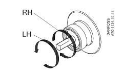
Note! Shaft rotation, location of nozzle outlet and other connections are seen from shaft end.
