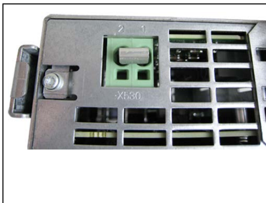
Terminal X530 with connector jumper
