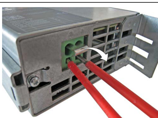
Relieve the springs and withdraw the connector jumper
