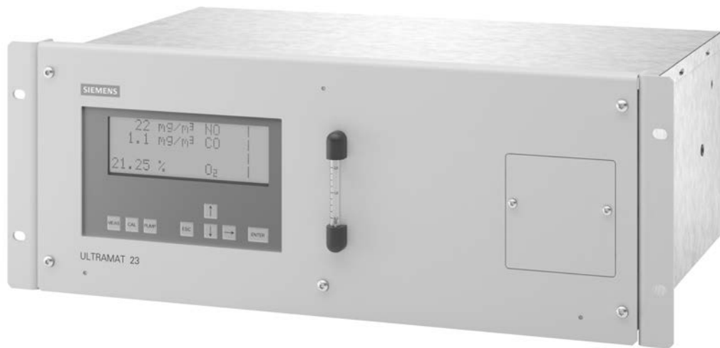
Figure 3-1 Front view of ULTRAMAT 23 for measurement of CO, NO, and O 2 (example of rack unit)
