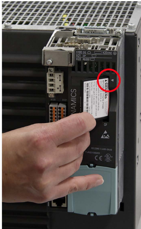
Figure 7-12 CU310-2 DP Inserting the memory card
