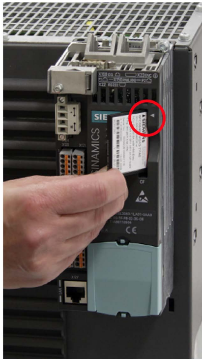
Figure 7-5 CU310-2 PN Inserting the memory card
