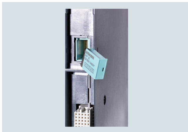
Plugging the C-plug into the rear of the CP 443-1 Advanced
