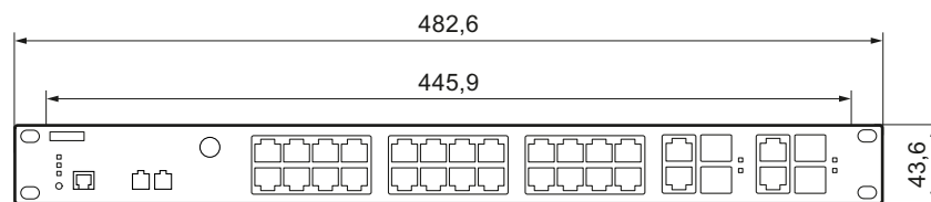
Figure 9-1 Width and height based on the example of a 24 V DC variant
