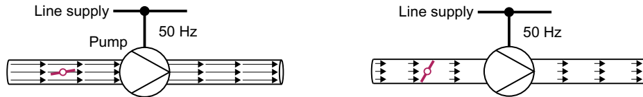
Figure 6-75 Flow control with pump and throttle connected to a 50 Hz line supply
