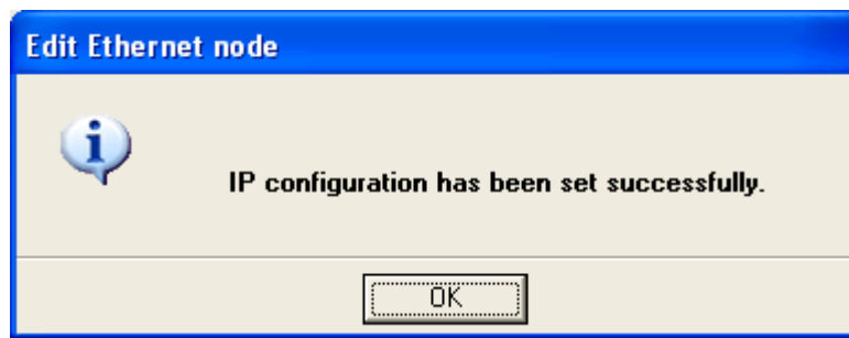
Figure 10-41 STARTER - Successful assignment of the IP configuration
