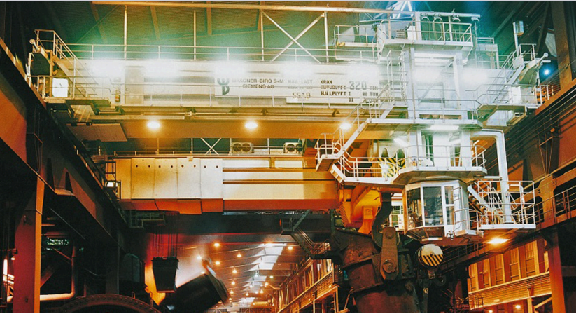
Example: Ladle crane, lifting capacity 200 - 500 t, gantry speed approx. 60 m/min
