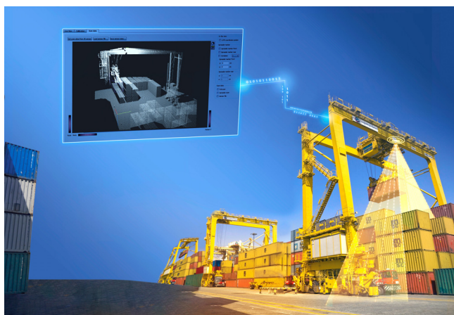
Example scene for load collision prevention RTG
