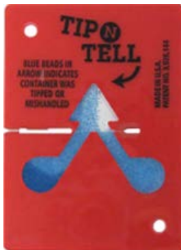
Figure 2-3 Tilt indicator tripped
