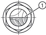
Figure 10-6 Oil level in the oil sight glass
