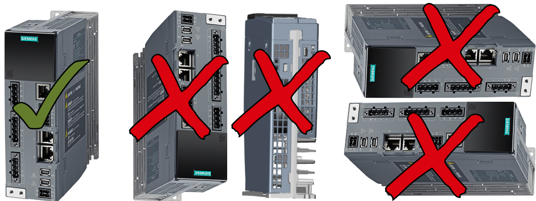
Figure 7-2 Mounting position of the converter
