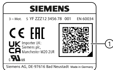
Figure 3-5 Conformity plate with ID link
