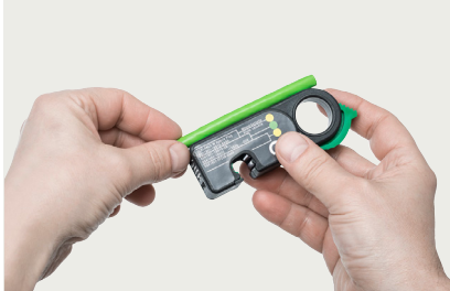
Measure the cable end
