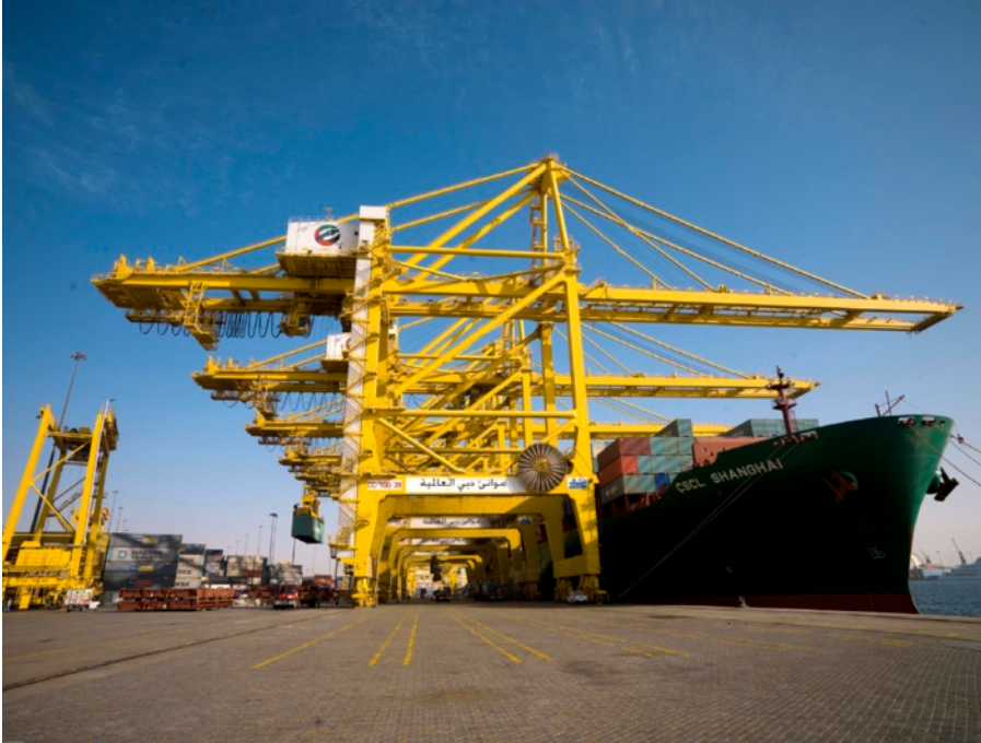
Example: STS crane, lifting capacity up to 120 t, trolley speed up to 250 m/min
