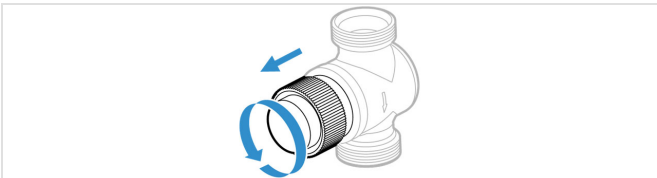
Fig. 2 Removing protection cap
