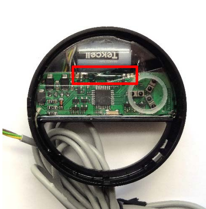
Figure 3. Position of reed switch in module EWA110C1520-MBUS and EWA110C2540-MBUS
