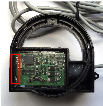
Figure 4. Position of reed switch in module EWA171C-MBUS
