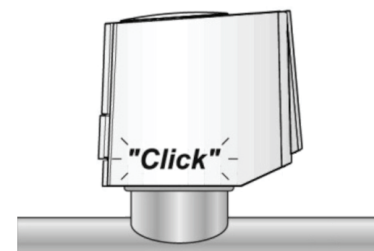
Fig. 10 Step 3: Pressing down actuator onto valve adapter
