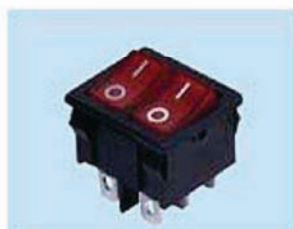
RSSM2101 ON-OFF 10 A 125 VAC; 6 A 250 VAC DPST 6P
