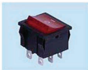
RSM2024 ON-ON 10 A 125 VAC; 6 A 250 VAC DPDT 6P
