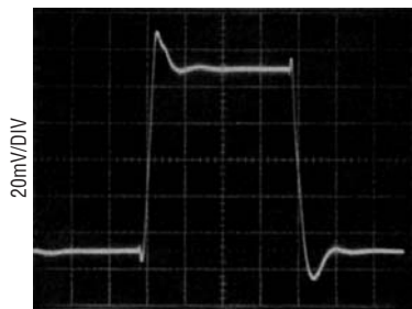
Small-Signal Transient Response V_S = \pm 2.5V
