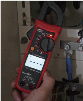
NCV multi-segment display and audio/visual alarm
