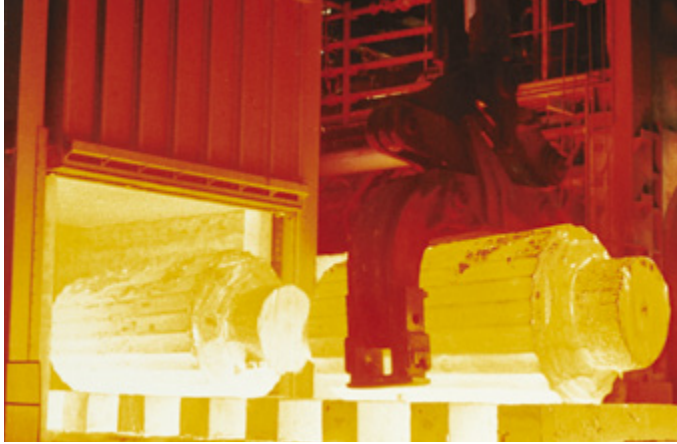
Metallurgical industry: forging furnace
