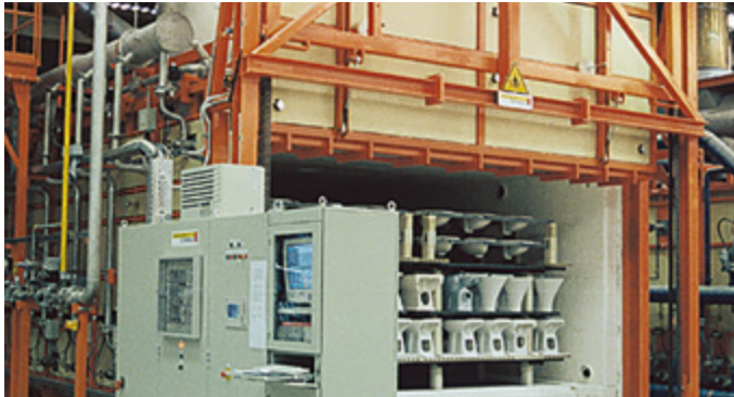
Intermittent shuttle kiln in the ceramics industry
